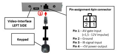
Connect the female 4pin connector of the keypad to the male 4pin connector of the video-interface.
