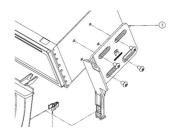
14. Place the stereo and bracket assembly into the dashboard, making all wiring connections, and screw into place using the OEM screws
