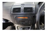
2. Disconnect the hazard switch and wiring to the air vents, and remove the vents
