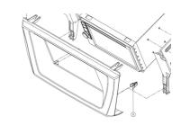
16. Place the climate control button assembly into the new hood and fix to the top of the dash.
