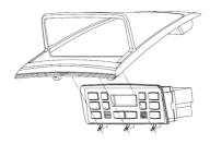
17. Finally reconnect the hazard switch, pushing it into place, to complete the installation.
