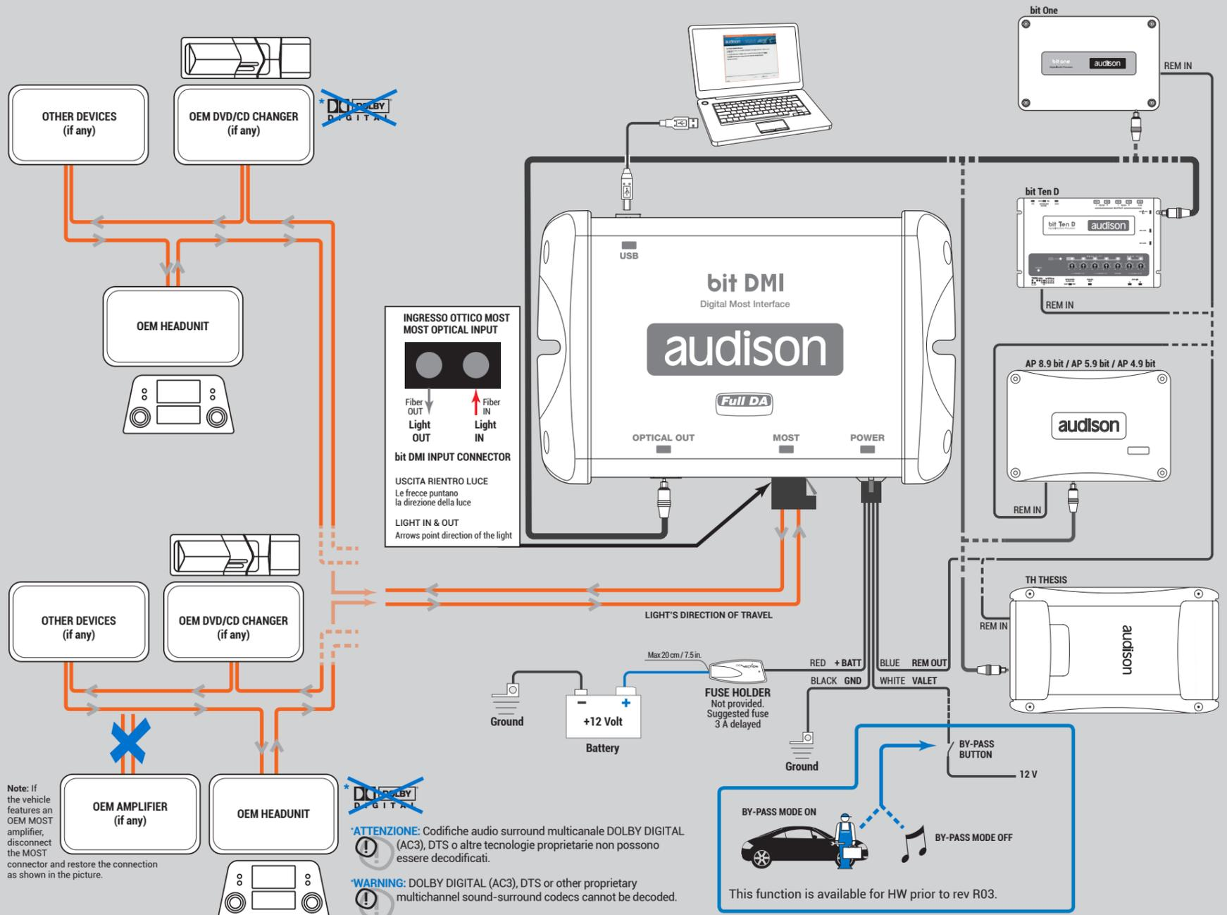
Note: If the vehicle features an OEM MOST amplifier, disconnect the MOST connector and restore the connection as shown in the picture.
