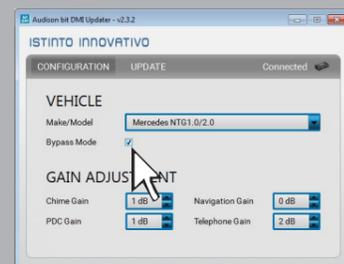
Flag "Bypass mode" only in the event of interventions in a garage, to exclude the audio system and any diagnostic errors.
