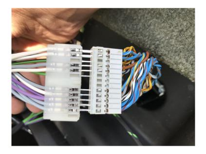
The above image shows how the connector on the 20-316 lead to the left mates with the original connector on the right.
